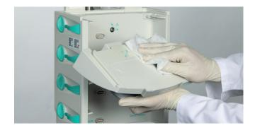
In case of heavy contamination remove cover – unlock the locking button and remove the SpaceCover. Remove visual contamination on the SpaceCover and the guide rail as described above. Dispose the cloth after usage.
