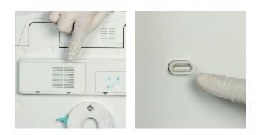
Make sure that no liquid is leaking into the ventilation or connectors. Let the SpaceStation time to dry after cleaning/disinfection. Afterwards assemble the SpaceCover again and lock it.
