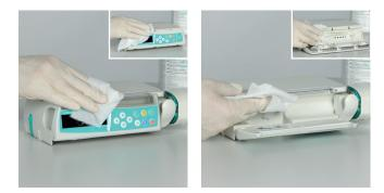
Clean/disinfect all sides of the Space Infusion pump. Start with the display and use ready-to-use wipes or a moistened fleece cloth. Clean with a moist, NOT a wet fleece cloth. Dispose cloth after usage.
