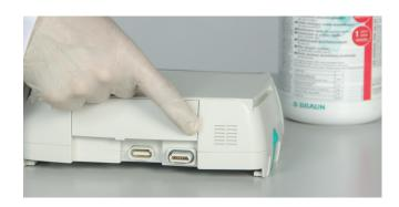
Make sure that no liquid is leaking into the ventilation or connectors. Let the device at least one minute to dry after cleaning/disinfection.
