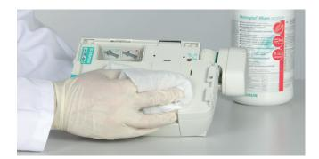
To clean the flexible cable of the the Infusomat<sup>®</sup> Space and of the Perfusor<sup>®</sup> Space we recommend Meliseptol<sup>®</sup> Foam pure. Clean with cotton carrier in use with lint-free tissue.
